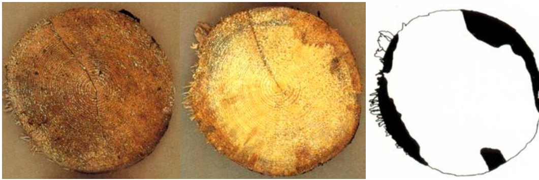
Figure 7. Storage decay in spruce. Left: end surface of the log; Middle: a cross-section 15 cm from the log end; Right: Storage decay highlighted in black. Log diameter 20 cm, 25% storage rot (Rötskador i massaved, Swedish Forest Agency, 1989).
